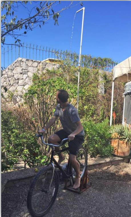
First bicycle pump prototype – pumping 3 meters high
